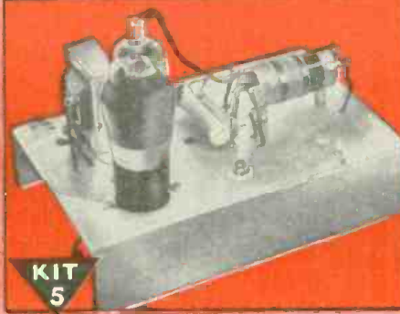
KIT 5 Building this A. M. Signal Generator gives you more valuable experience. It provides amplitude-modulated signals for many tests and experiments.
